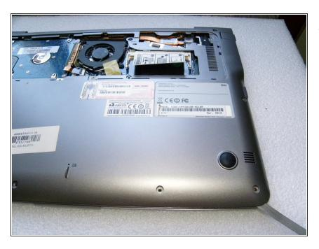
Ensure that the hard disk has been removed. Carefully detach the bottom cover.
