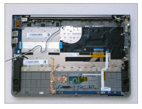
To remove the Motherboard, carefully disconnect the cables.
