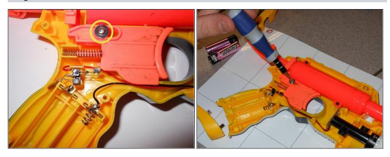
• Remove the phillips head, 10.2 mm screw holding the trigger in place.
