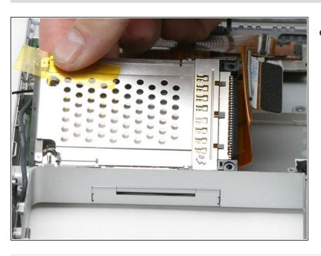
Lift the PC card cage up from the front, and remove it from the computer.
