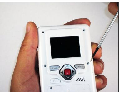
Remove the 5 10mm screws with the #00 Phillips screwdriver. These connect the back of the outer shell to the front of the outer shell.
