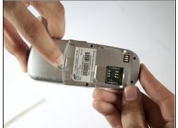
Remove the battery by pressing down on the battery release button while sliding the battery downwards.
