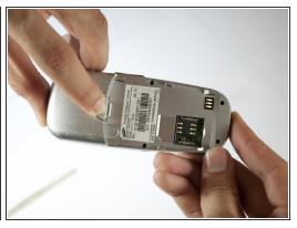
Remove the battery by pressing down on the battery release button while sliding the battery downwards.
