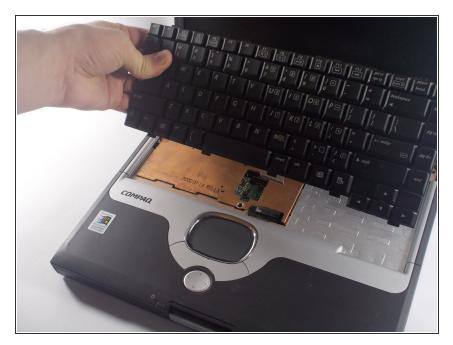
Pull the keyboard upward to remove it from the device.
