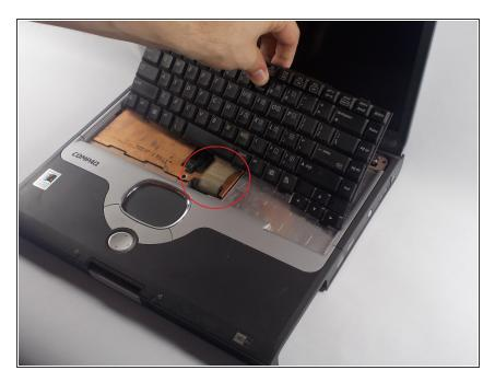
Pull the keyboard slightly toward the screen of the device to reveal the connecting cable below.
