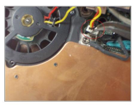
Remove the cable with the grip tweezers as shown in the photo.
