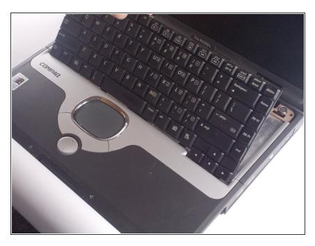
Lift the keyboard up from the back end as shown in the image.
