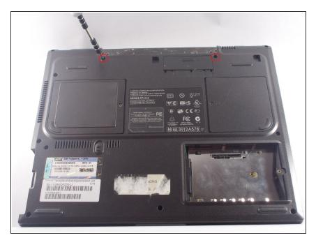
Carefully remove the screws located inside the red circles.
