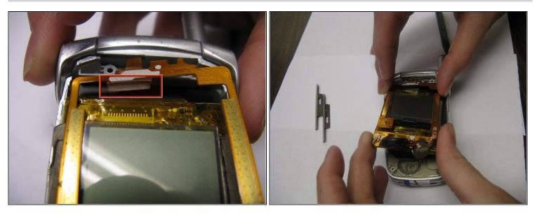
• With the copper screen lifted up, gently pull out the ribbon connector and lift out the LCD screen.
