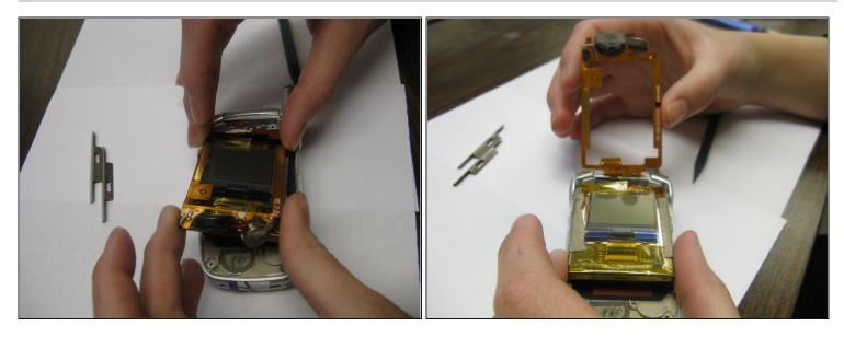
$\triangle$  The copper frame is attached to the phone at the hinge. Do not tear the frame.
