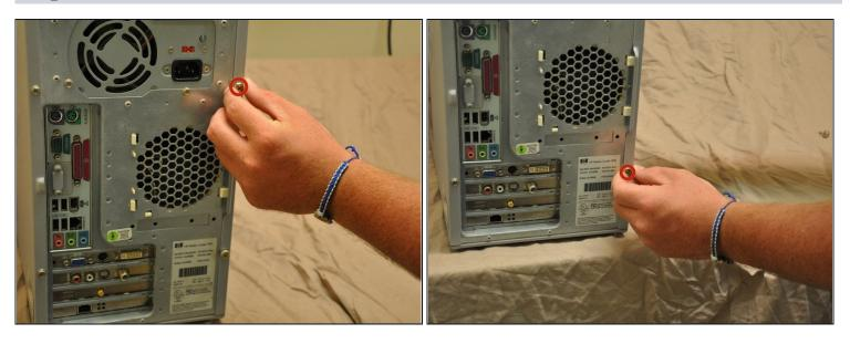
Remove the two (9 mm) hand screws on the back panel.
