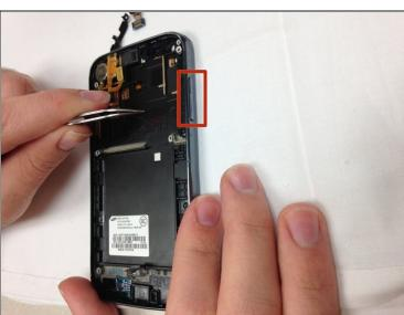
Lift the tab indicated by the red rectangle using a pair of tweezers.
