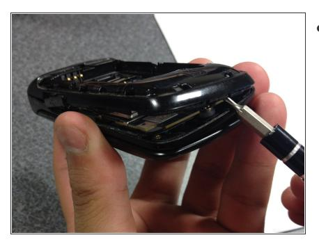
• With tweezers, pry around the sides to expose the circuitry.
