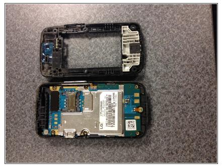
• Remove the back part of the phone to expose the layers inside.
