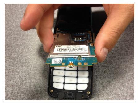
• Remove the layer connected with the keypad.
