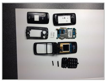
• Remove all loose part, and should result in the components shown in the picture.
