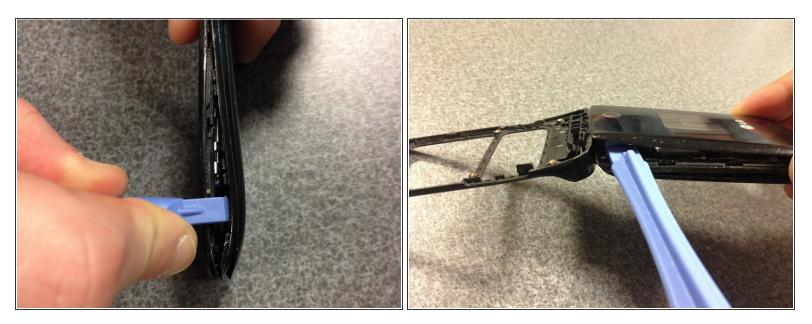
• With a prying tool, start opening the front face of the phone.
