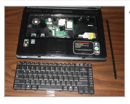
Remove the keyboard completely from the laptop. To reassemble your device, follow these instructions in reverse order.
