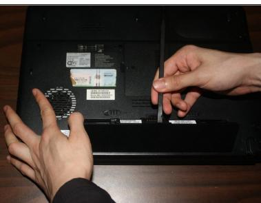
While holding the left battery lock to the left, lift up the battery using the tab located on the top center of the battery.
