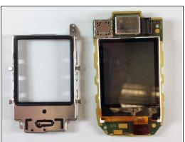
If the metal case is not already free, simultaneously release the metal tabs on both sides of the metal casing to remove the display screen.
