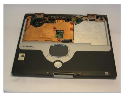
• Remove the four screws from the heat sink.
