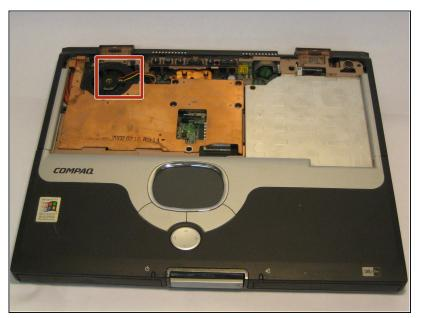
Disconnect the cable connecting the fan to the system board.
