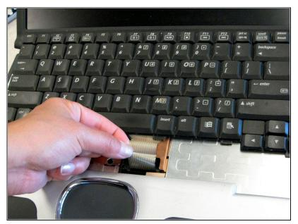
• Pull the cable and lift up to release.
