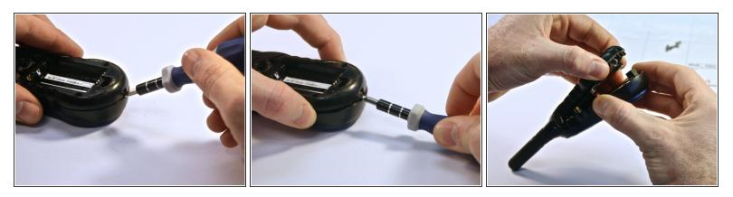
Gently open the backplate of the radio. Use a flathead screwdriver to slowly pry apart the two sides.
