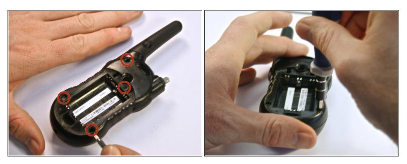
Remove the four 3 millimeter T8 Torx screws from the back of the radio.
