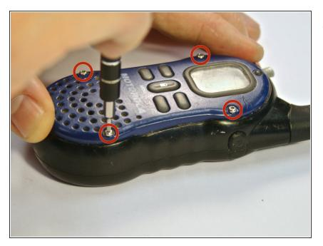
Remove the four 3 millimeter T6 Torx screws from the front of the radio.
