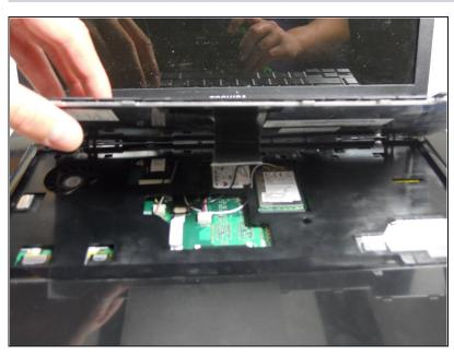
With the black ribbon cable now disconnected, remove the keyboard from its housing.
