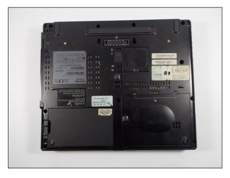
Use a Phillips screwdriver to remove the two screws securing the hard driver cover.
