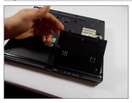
Gently lift the plastic cover from the back case and slide it out from its position.
