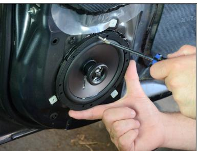
Use a #2 Phillips screwdriver to hand tighten the top mounted screw. Do not use a drill or power driver for this task -- you'll have a bad time if you strip the hole.
