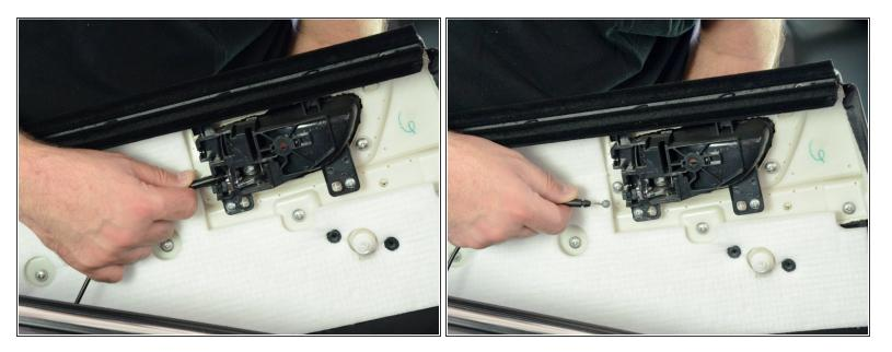
Repeat the same procedure above with the black cable. First disconnect the black sleeve, then the ball, and finally move the entire cable away from the door panel.
