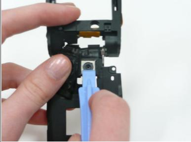
Push metal camera cover through the hole to remove camera.
