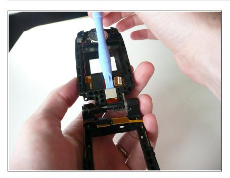
Use iPod opening device to remove the metal cover.
