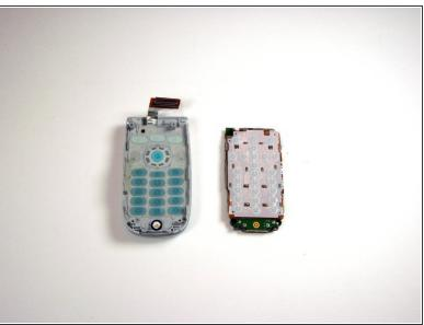
Use a flathead screwdriver to gently pry the logic board and keypad from the device.
