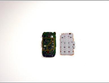
Peel the keypad from the logic board using your thumb.
