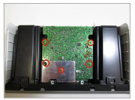
Unscrew at the marked points with #2 Phillips screwdriver.
