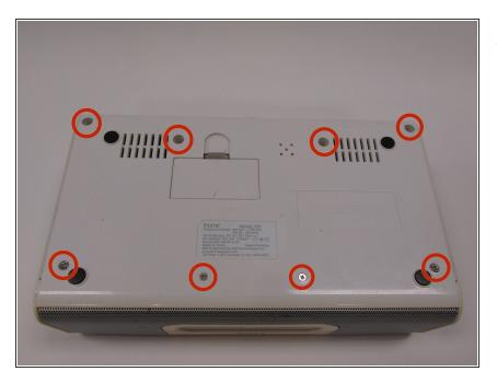
Unscrew the bottom of the iHome at the marked points with a #2 phillips
