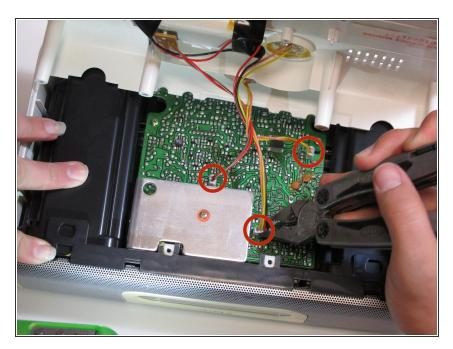
Remove wires from the logic board (tweezers or pliers are helpful)
