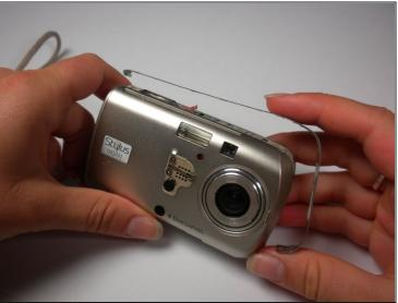
• Use the spudger to peel off the outer metal band, starting from the bottom of the camera.
