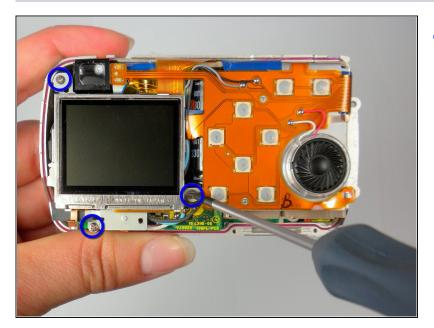
Locate the 3 internal screws holding on the front of the case. Remove them with a #00 Phillips screwdriver.
