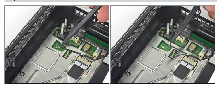
• Use the tip of a spudger to disconnect the antenna cable from the motherboard.
