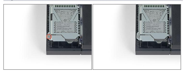
• Use a Phillips screwdriver to remove the 6.5 mm screw securing the hard drive bracket to the enclosure.
