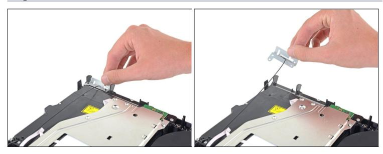
Remove the Wi-Fi antenna.
