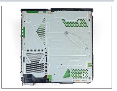
Remove the twelve 9.7 mm Torx screws securing the upper EMI shield.
