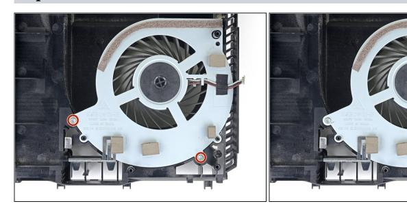
• Remove the two 6.2 mm Phillips screws from the fan.
