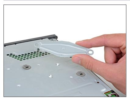
• Remove the pressure plate.
