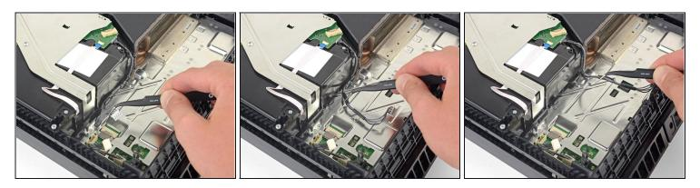
• Use your fingers or a pair of tweezers to remove the optical drive cable from the cable guides that hold it in place.
