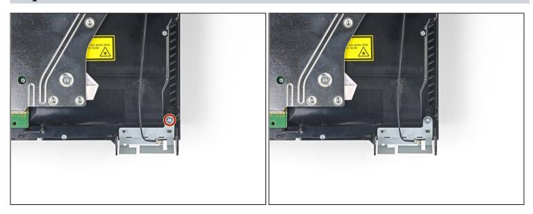
• Remove the 9.7 mm Torx security screw securing the antenna.
