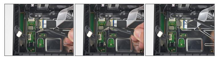
• Use a pair of <u>tweezers</u> or your fingers to grab the antenna cable and move it out from the cable guides.
