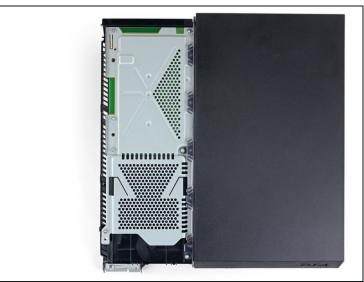
• Remove the two 9.7 mm Torx screws securing the upper case.
