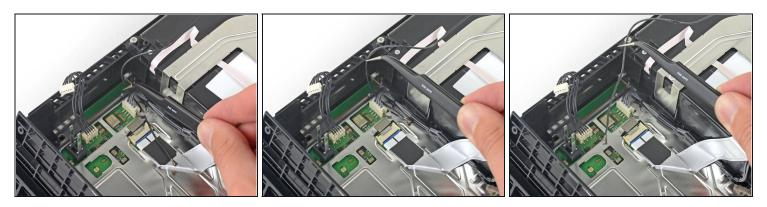
• Use a pair of tweezers or your fingers to thread the antenna cable out from underneath the optical drive cable.
