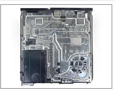
• Remove the three 6.2 mm Phillips screws from the lower EMI shield.
