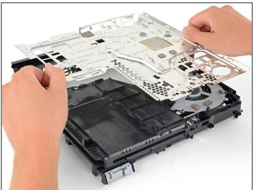
• Lift the lower EMI shield and heatsink straight up out of the PS4.
