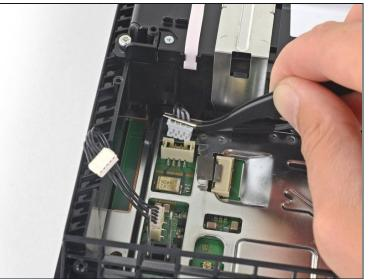
Use your fingers or a pair of tweezers to disconnect the optical drive cable from the motherboard.
