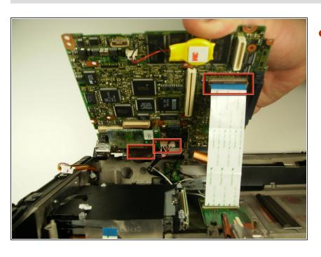
Detach the white ribbon cable, the white cluster connector, and the ribbon cable right next to the cluster
