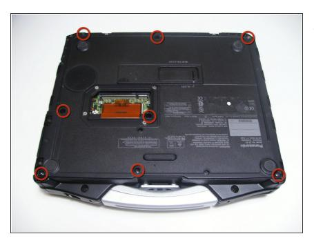
Use a Phillips size 1 screwdriver to remove the remaining 8 screws.
