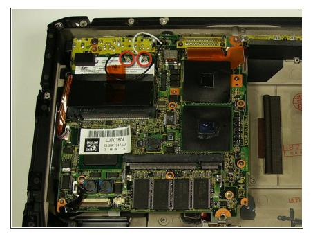
Remove the black and white wires attached to the wireless card by simply pulling up.
