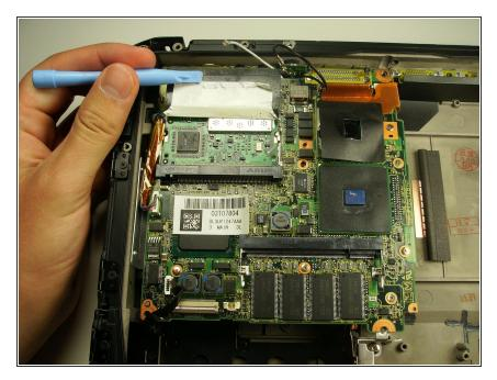
Peel back the black cover to expose the clips holding in the wireless card.
