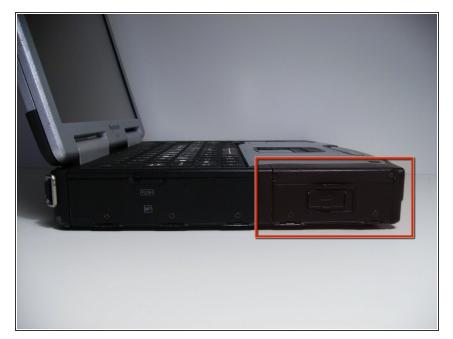
Locate the bay door for the battery on the left side of the laptop.
