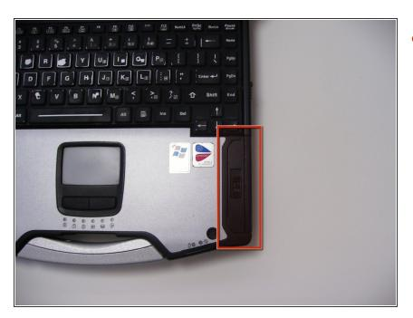
Locate the door for the hard drive on the right side of the laptop
