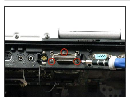
On the back of the unit, unscrew the three screws surrounding the serial port.
