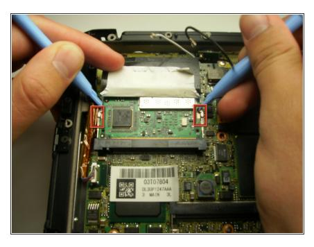
Using a pair of plastic opening tools, push the two metal tabs away from the card.
