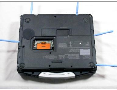
Use a plastic opening tool to release, but NOT remove, the back cover because it is sealed with adhesive.
