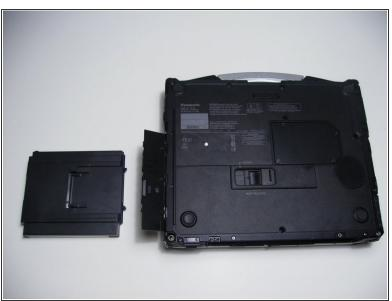
Push the exposed switch to the left to eject the optical drive.
