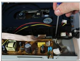
Remove the four 8.1mm screws in each of the corners of the disc tray.
