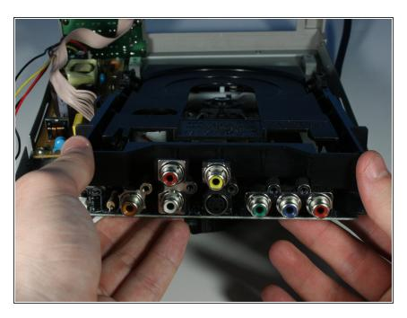
Orient the device so the back is facing towards you. Remove the disk tray out towards the back of the DVD player by lifting it.
