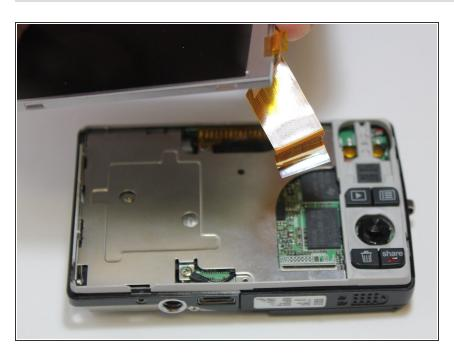
Lift LCD Screen off of device.
