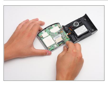
Once the two covers are separated, use the tweezers, or even your fingers, to gently disconnect the two sets of wires that are connected to the motherboard from the back cover. You may have to wiggle the wires a little bit to get them to disconnect.
