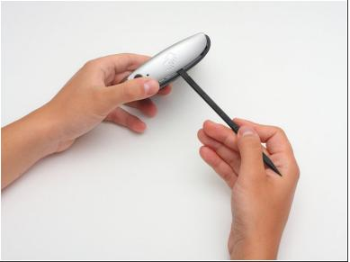
Using the spudger, gently pry apart the back case from the front case. It is easier to start on a side and work your way around the device.
