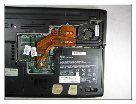
Remove the four 9 mm Phillips #0 screws from the cooling assembly.
