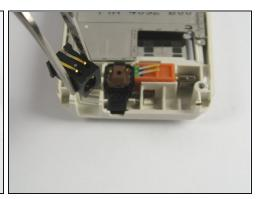
• Use a pair of <u>tweezers</u> to remove the DC input from the base.
