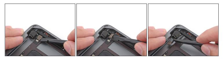
• Use the flat end of a spudger to disconnect the rear-facing camera connector from the logic board.
