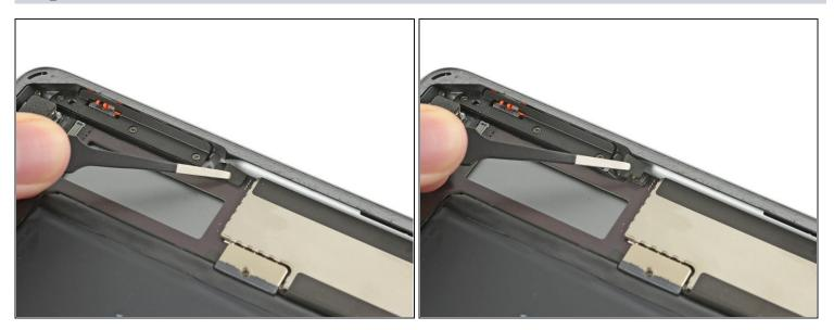
• Remove any tape covering the upper button assembly cable connector.
