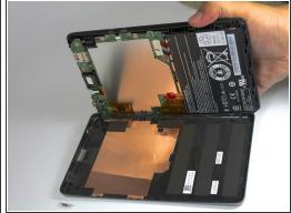
Pry open the left side of the case with a plastic opening tool. The backside of the tablet should now separate completely from the front.
