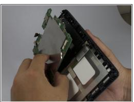
After all ribbon cables are disconnected, move them out of the way, and the motherboard should fall out easily.
