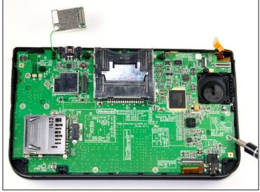
• Remove ten 3.0 mm screws that are located around the face of the motherboard.
