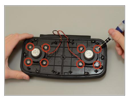
Remove the four 6mm screws that hold the broken speaker in place.
