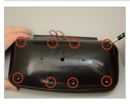
Remove these eight 9 mm screws using a Phillips #2 driver.
