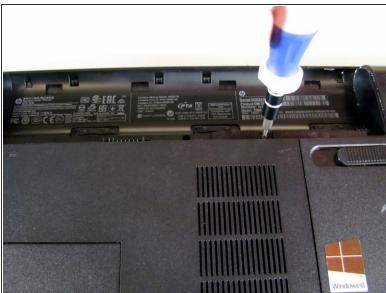
• Loosen the Phillips #00 screw securing the RAM compartment cover.
