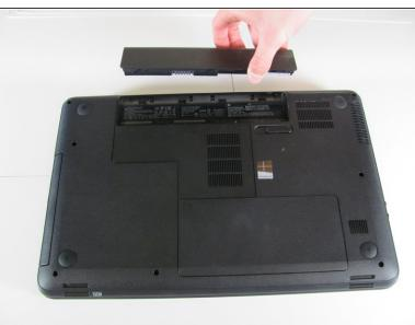
Slowly pull the battery out of its slot, being careful not to damage any of the connectors in the process.
