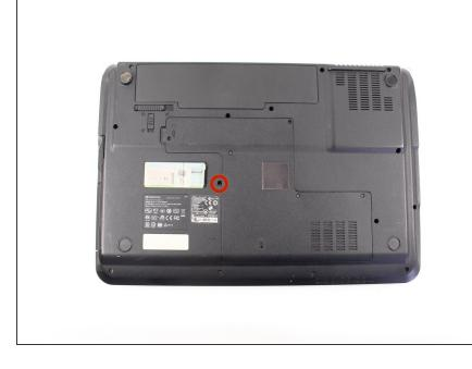
Remove the single 3/16" screw with the Phillips #0 Screwdriver that secures the Optical Drive.
