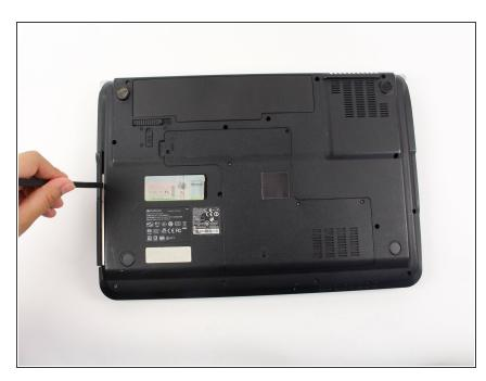
Slightly wiggle the Optical Drive from the laptop using the Heavy Duty Spudger.
