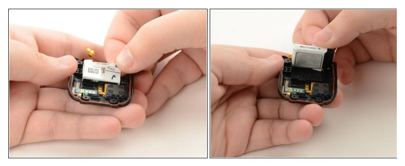
• Remove the battery by pulling the white tab on the battery marked "PULL."
