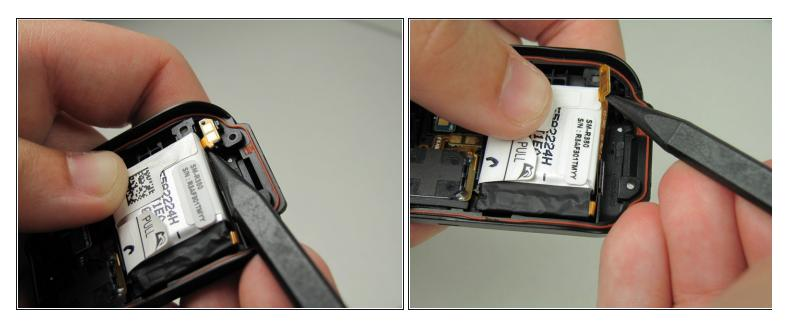
• Use the pointed side of the spudger to remove the small, orange battery cable.
