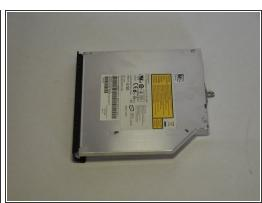
Push the Optical Disk Drive out using a spudger tool as shown and pull from the front cover of the Optical Disk Drive.
