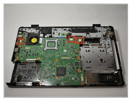
Disconnect the Thermal Fan cable,
