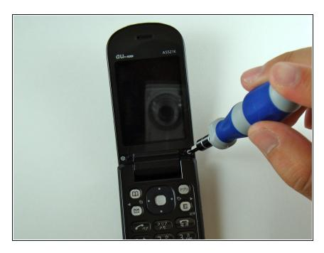
Remove the screws using a Y0 screwdriver.
