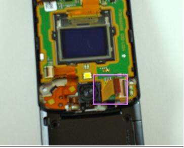
Firmly grab the flexible circuit with tweezers to detach (or use your fingers if you can manage a firm grip).
