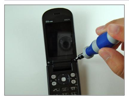
Remove the screws using a Y0 screwdriver.
