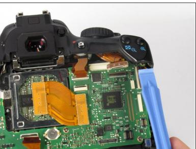
• In the upper right corner of the motherboard, use the plastic opening tool to remove the clear cable connector from the motherboard.
