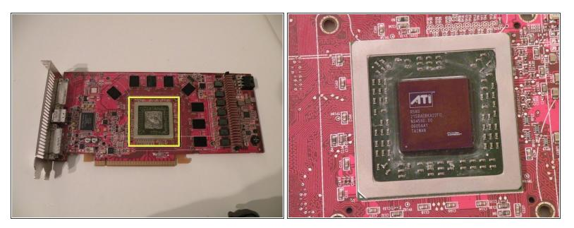
• Using the same method that you used to clean the copper plate, clean the surface of the GPU die.
