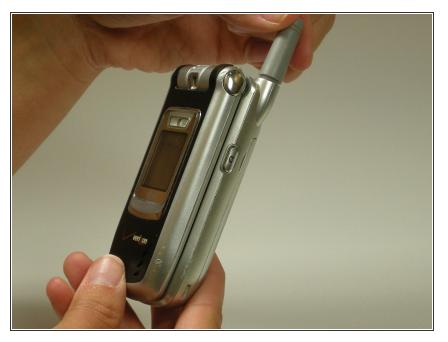
• Remove existing antenna, if any, by unscrewing counterclockwise.
