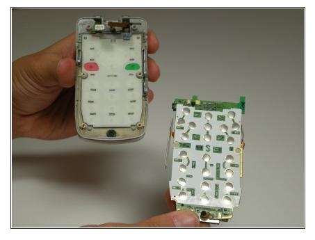
• Insert replacement keypad with buttons aligned in proper holes.
