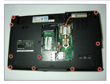
Remove the 11 screws (5mm Phillips #1) from the back of the laptop as marked. One screw is in the middle, by the RAM.
