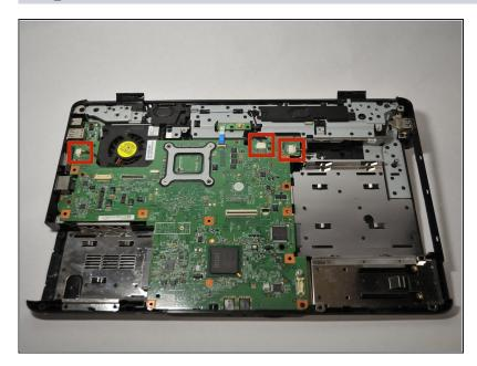
Disconnect the Thermal Fan cable, Speaker cable, and USB Board cable from their connectors.
