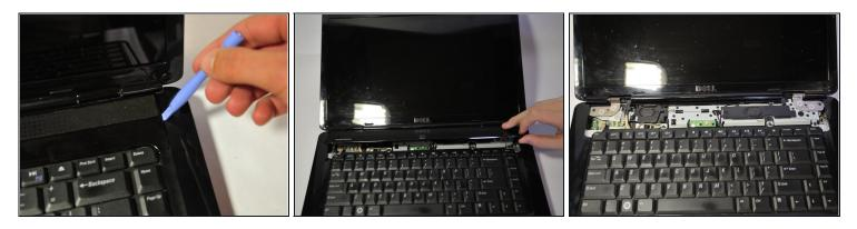
A The Center Control Cover is VERY fragile, be careful when using prying tools.
