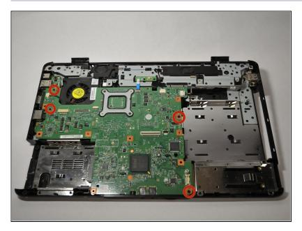
Remove the two screws (3mm, Phillips #1) on the left and the two screws (5mm, Phillips #1) on the right that secure the Motherboard to the laptop.
