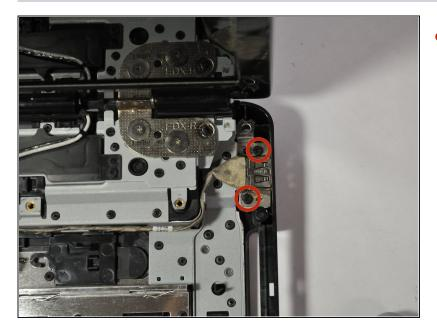
• There is another USB board on the right side of the laptop. To remove this simply remove the two screws (5mm, Phillips #1) and lift the port up.
