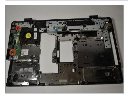
Remove the two screws (5mm, Phillips #1) in order to remove the main auxiliary board containing USB ports, and audio/microphone ports.
