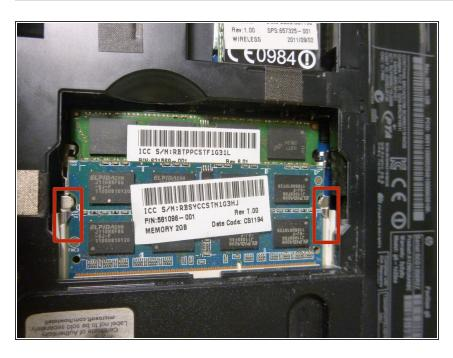
Move the two tabs outward to release the RAM stick, then pull it out. Repeat for the other stick.
