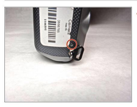
Remove the 3.25 mm exterior screw with a Phillips screwdriver.
