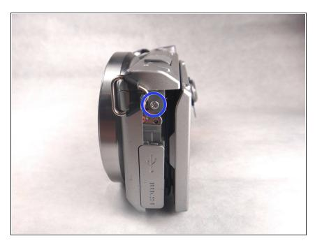
Remove the 3.5mm phillips head screw on the top left of the camera.
