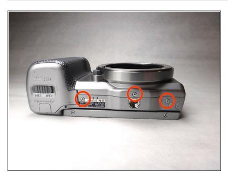
Remove the three (3.5 mm) screws from the bottom of the camera with the Phillips screwdriver.
