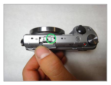
Remove the 3.5mm phillips head screw underneath the flash port
