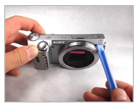
Use the spudger tool to go around the seam of the top panel. The top should easily lift off.
