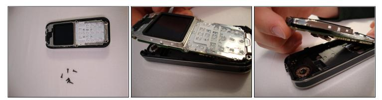
• Lift the logic board and screen from the top.
