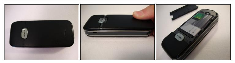
• Press down on the grip on the back of the phone and slide the rear housing down towards the bottom of the phone.
