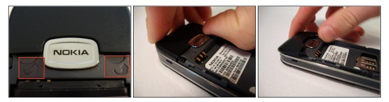
• Insert your two fingers under the two tabs found at the top of the phone underneath the black casing, then pull the casing up and slide it out slowly.
