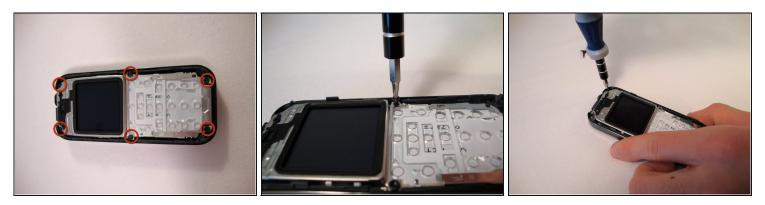
• Remove the six screws with a T-6 Torx screwdriver.
