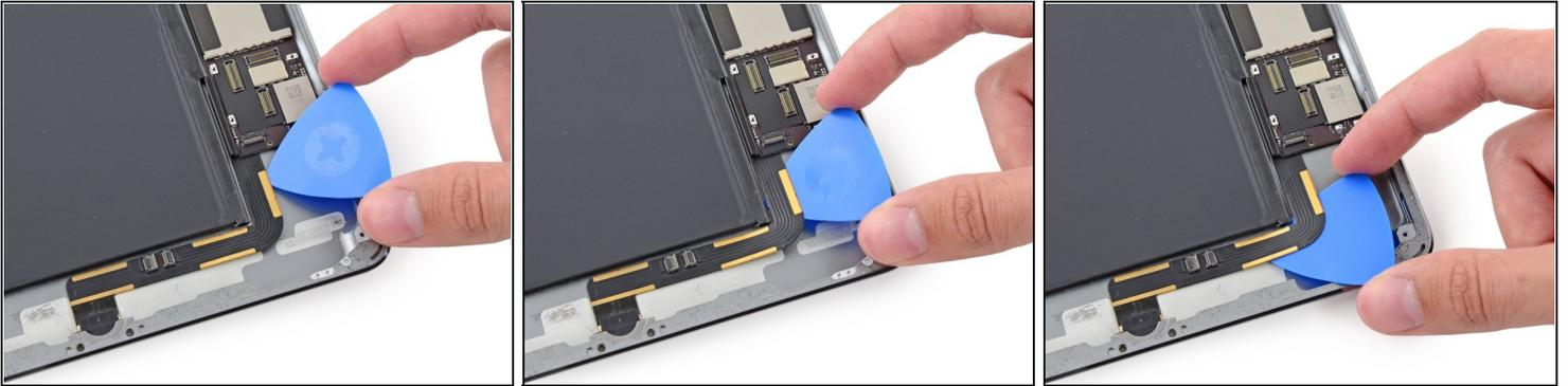
ⓘ The Lightning connector cable is stuck to the case with some adhesive. To detach the adhesive you will be sliding an opening pick between the cable and the case. **Be very careful** not to cut the Lightning connector cable itself.
