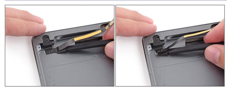
• Continue to slide the spudger under the end of the headphone jack cable to remove the last of the adhesive.
