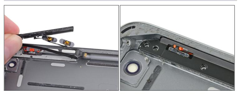
• Lift the button assembly carefully out of the rear case.
