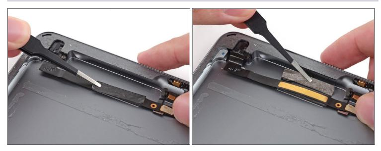
• Lift the tape covering the headphone jack cable toward the top of the iPad to free the cable for removal.
