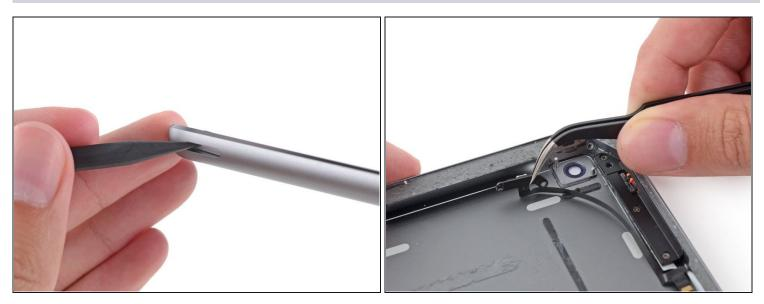
• Use the tip of a spudger to push the power button into the rear case from the outside.
