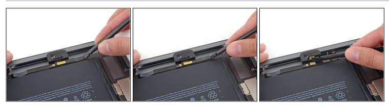
• Use the flat end of a spudger to disconnect the front-facing camera connector from the logic board.
