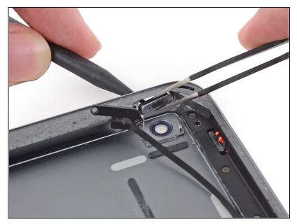
• Push the power button into the case and remove it from the iPad.
