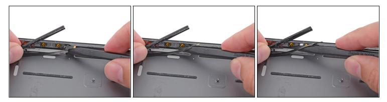
• Slide the point of a spudger under the ribbon cable near the button cables to free it from the adhesive holding it to the rear case.
