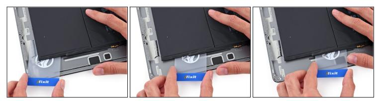
• With the card roughly halfway inserted, slide it toward the top of the iPad, stopping before the battery contact post.
