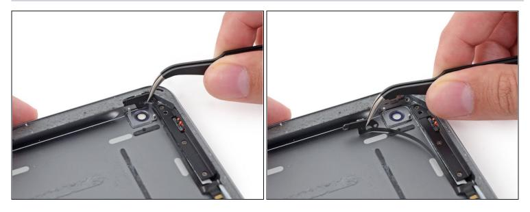
• With the power button cable bracket loosened, peel it off of the rear case with a set of <u>tweezers</u> and move it out of the way.
