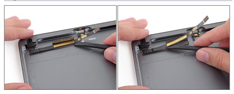
• Slide the flat end of a spudger under the headphone jack cable to free it from the adhesive securing it to the rear case.
