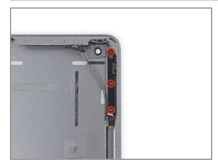
Remove the three 2.3 mm Phillips #000 screws from the button cable bracket.
