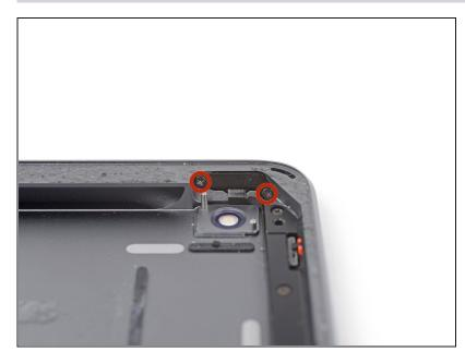
Remove the two 2.3 mm Phillips #000 screws from the power button cable bracket.
