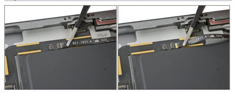
• Slide the speaker cable straight out of its ZIF connector.
