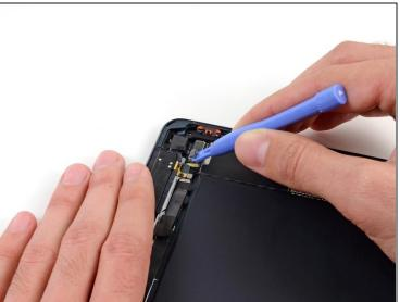
• Use a plastic opening tool to pry the top right antenna ribbon cable up from its socket on the logic board.
